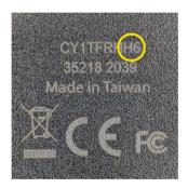
Updated Firmware Notation marked as JA or H6 – marked on the backside of the CFexpress™ Memory Card
